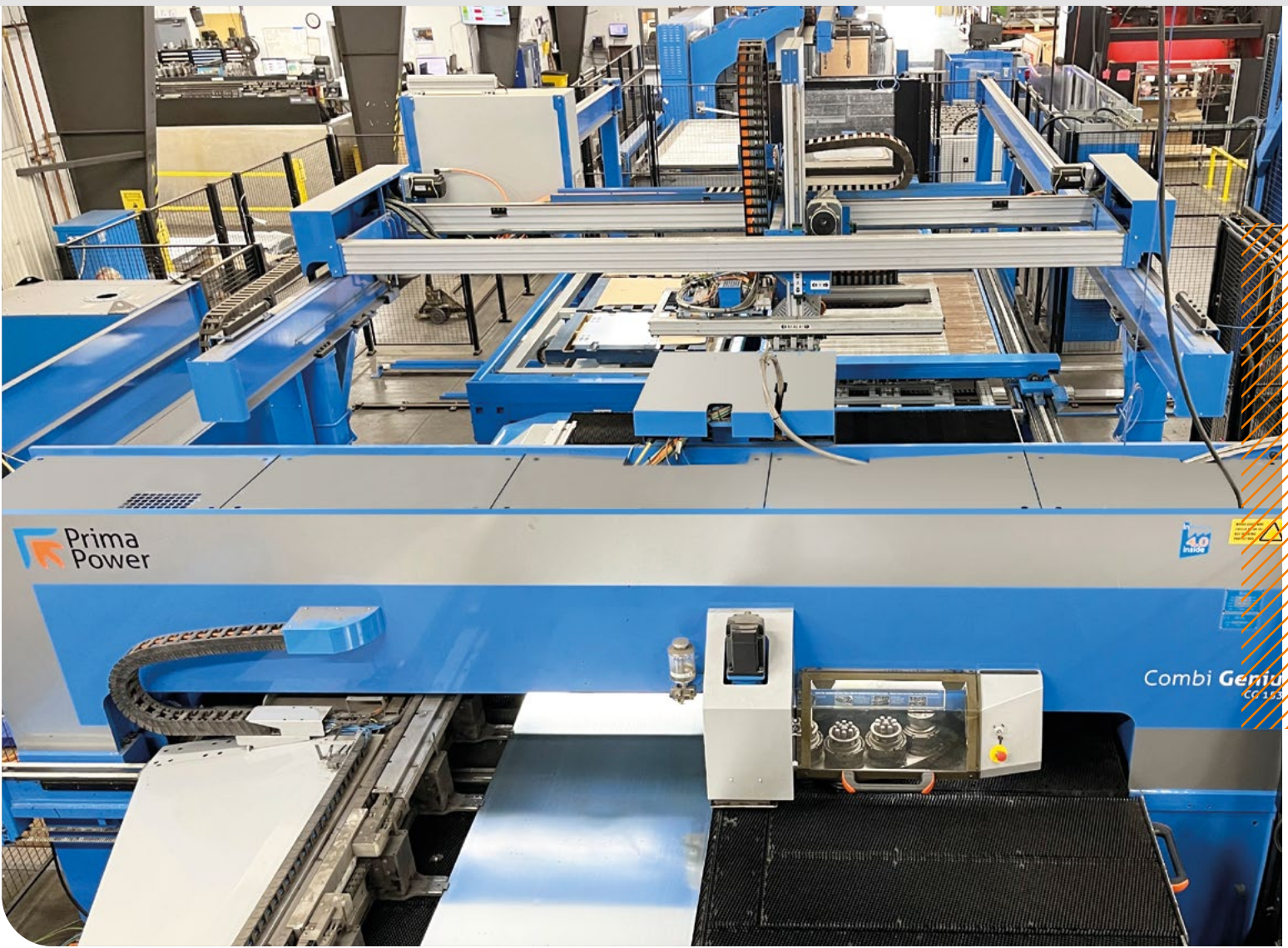
The Combi Genius punching and laser cutting integrated cell combines servo-electric and fiber laser technologies into a fast, accurate automated solution with one setup.
